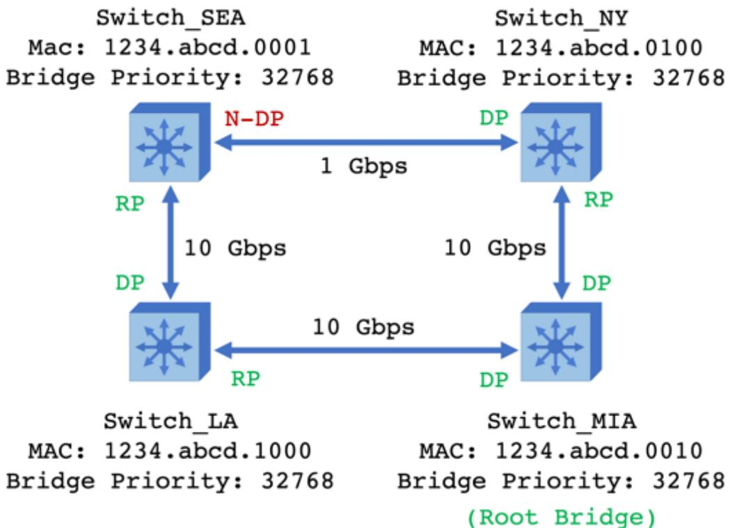
24. In this example, refer to the diagram below and use the Command Line Interface (CLI) on each switch to determine which switch is the Rapid Spanning Tree Protocol root bridge on VLAN 1:
