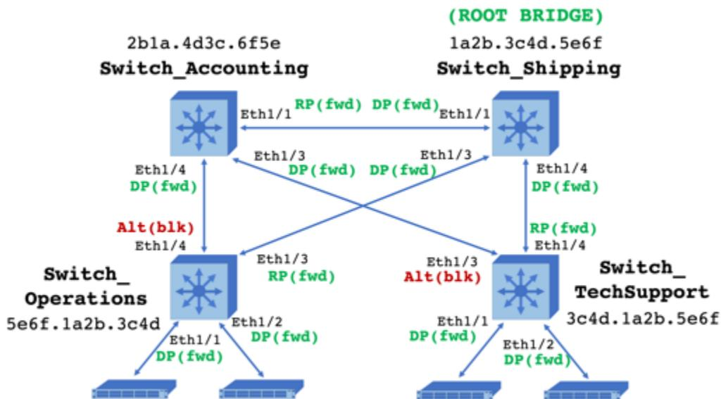
Switch\_Shipping is the root bridge and its Ethernet 1/1, Ethernet 1/3, and Ethernet 1/4 interfaces are designated ports in RSTP and will be forwarding frames.
