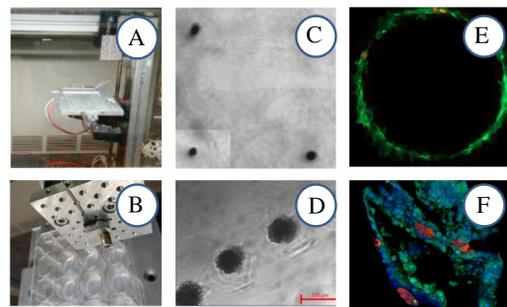
**Figure 1 (left):** Custom Bioprinter and printing applications. A) Bioprinter, into which can be loaded well plate and micro-extruder. B) Custom Bioprinter extruding bio-ink into gel, mid-print. C) Grid layout of MDCK cell spheroids. D) Arrayed Pan-02 spheroids, immediately post-print. E) Matured chimeric ring organoid composed of MCF-12A and ERBB2 cells. F) Histological slide of chimeric, 3D bioprinted structure composed of EPH4 and ERBB2 cells.
