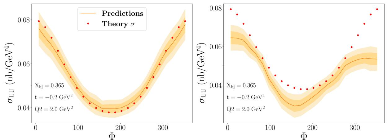
Figure 2 : DVCS generalization on kinematics outside of the range covered by the training samples. Left is the results using PINNs, right shows the results using basic NNs without physics knowledge incorporated.
