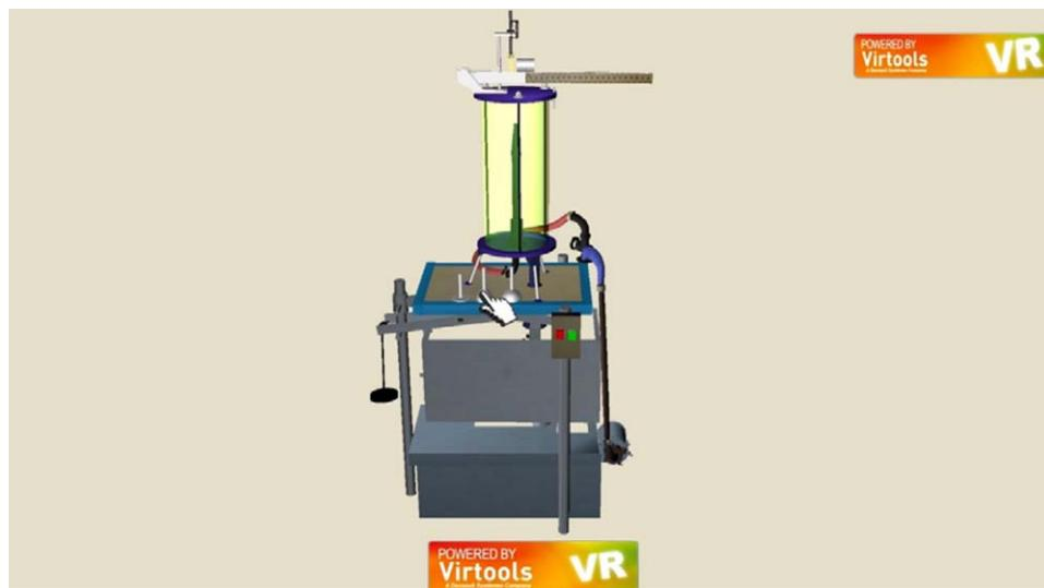
**Figure 7.** The Jet Force Experiment interface.
