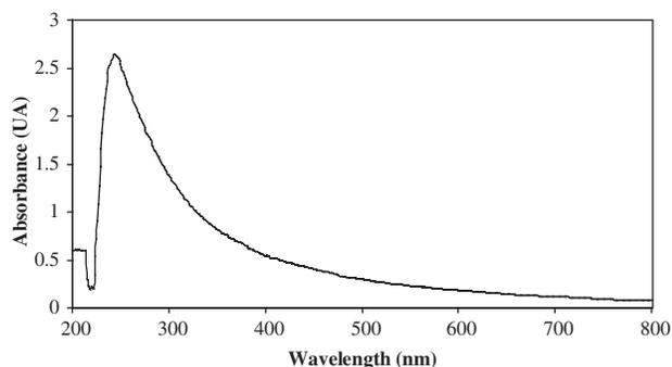
**Figure 2:** UV-sis spectrum of BNNT dispersion.
