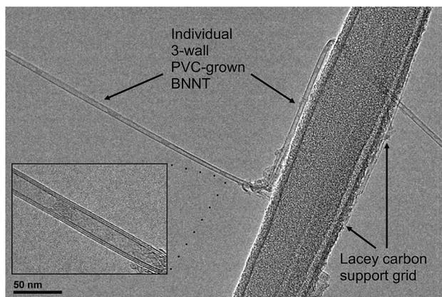
**Figure 1:** High resolution TEM image of an individual 3-wall PVC-grown BNNT.
