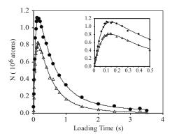
FIG. 2. Number of atoms as a function of loading time in a cw ( $\bullet$ ) and a pulsed ( $\triangle$ ) FORT for 7 W of FORT laser beam power,  $-8\Gamma$  MOT laser detuning,  $18.0~\mu\text{W/cm}^2$  repump laser intensity, and  $23.1~\text{mW/cm}^2$  trap laser intensity.
