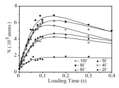
FIG. 5. Number of atoms as a function of loading time in a pulsed FORT for different trap laser detunings at 7 W FORT laser power, 13.1  $\mu$ W/cm<sup>2</sup> repump laser intensity, and 23.1 mW/cm<sup>2</sup> trap laser intensity.
