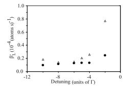
FIG. 7. Loss rates vs trap laser detuning in a cw ( $\bullet$ ) and a pulsed ( $\triangle$ ) FORT for 7 W FORT laser power 13.2  $\mu$ W/cm<sup>2</sup> repump laser intensity and 23.1 mW/cm<sup>2</sup> trap laser intensity.
