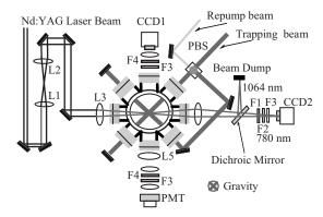
FIG. 1. The experimental setup for a cw and a pulsed FORT. L1=100 mm and L2=200 mm. F1=neutral density filter, F2=colored glass filter, F3=interference filter, and F4=short pass filter. PBS=polarizing beam splitter, PMT=photomultiplier, and CCD=charge coupled device camera.
