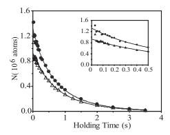
FIG. 3. Number of atoms vs holding time in a cw ( $\bullet$ ) and a pulsed ( $\triangle$ ) FORT for 7 W of FORT laser beam power,  $-8\Gamma$  MOT laser detuning,  $18.0 \ \mu\text{W/cm}^2$  repump laser intensity, and  $23.1 \ \text{mW/cm}^2$  trap laser intensity.
