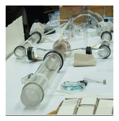
**Fig. 1.** Flexible Dual Port Olfactometer. This measuring instrument is designed to observe and document mosquito behavior. Note important component parts: staging area, stem or midpiece (flexible portion), and left and right arms for the placement of control agent and treatment odorant. The olfactometer was built to specification for Bernadette A. Ferraro by Scientific Glass, Virginia.
