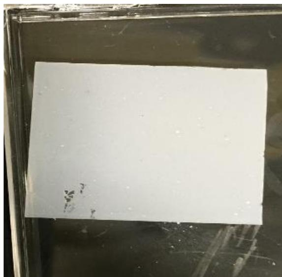
*Figure 14: Nitric acid treated BNNT spray deposition*
