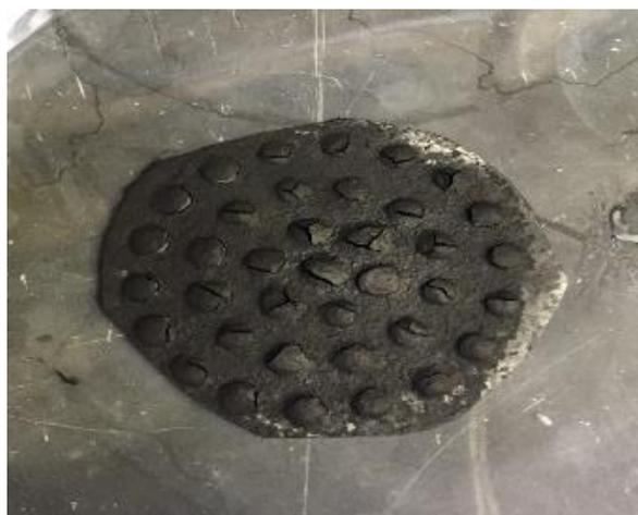
*Figure 15: CNT mat after vacuum filtration*
