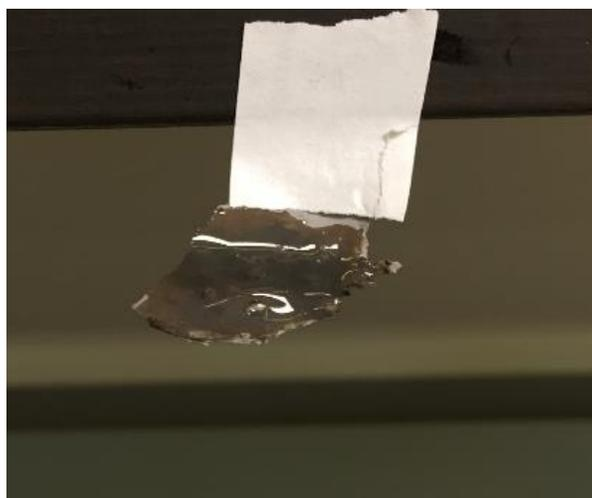
*Figure 22: BNNT mat coated with electrolyte gel*
