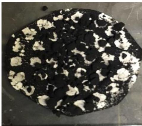
*Figure 16: CNT mat after drying*
