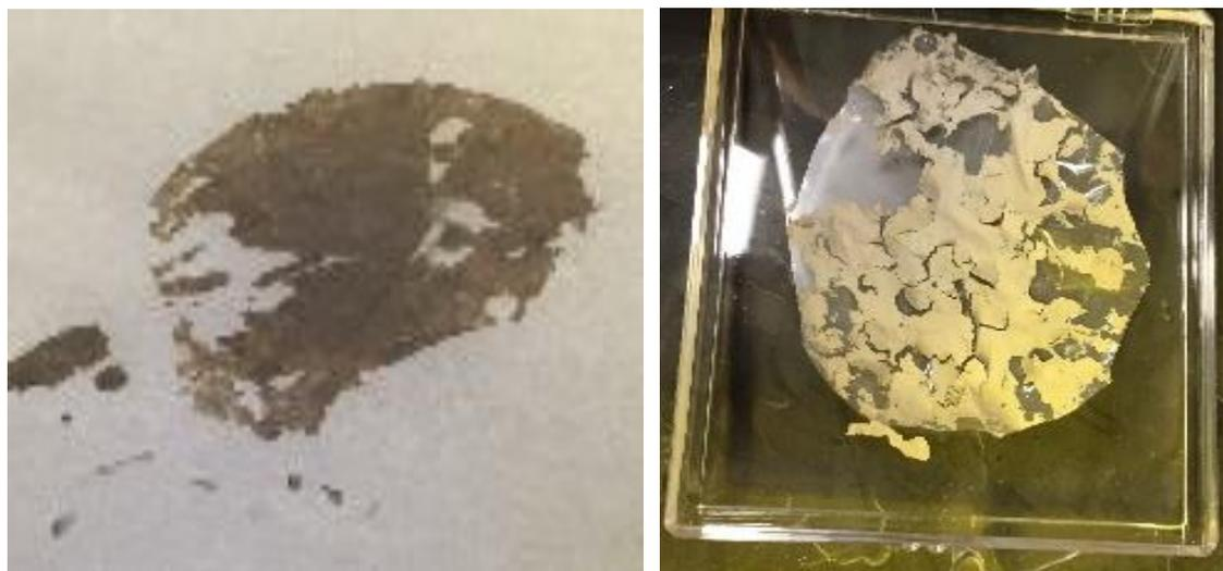
*Figure 8: Initial BNNT deposition on parchment paper (left) and PCTE membrane (right)*
