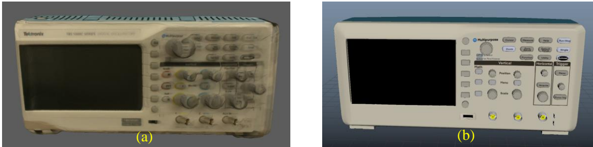
Figure 1. (a) Oscilloscope model generated by the Structure Sensor (b) Final 3D model.
