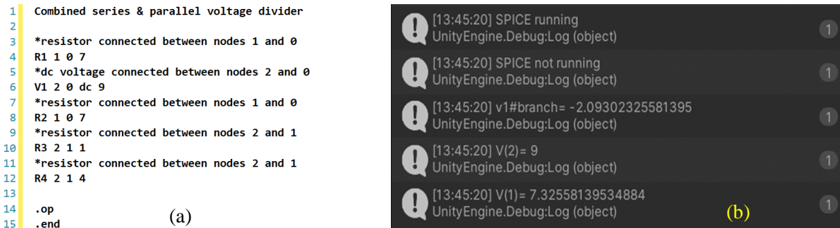
Figure 3. (a) The SPICE script generated from the circuit. (b) The simulation output.
