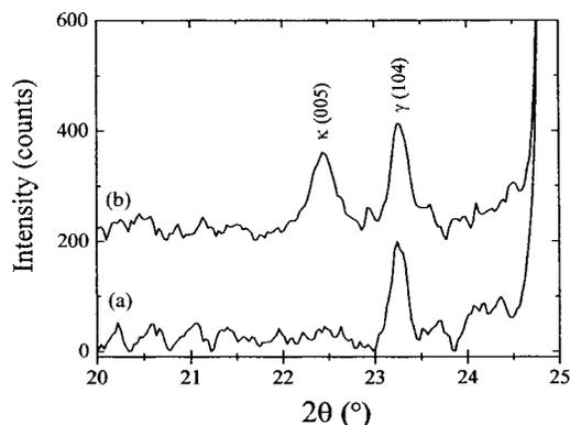
FIG. 6. Appearance of the diffraction peak (005) of the  $\kappa$ - $\text{In}_2\text{Se}_3$  phase in the x-ray diffraction pattern of the Zn doped  $\text{In}_2\text{Se}_3$  (b). (a) X-ray diffraction diagram of undoped  $\gamma$ - $\text{In}_2\text{Se}_3$  elaborated in the same conditions.
