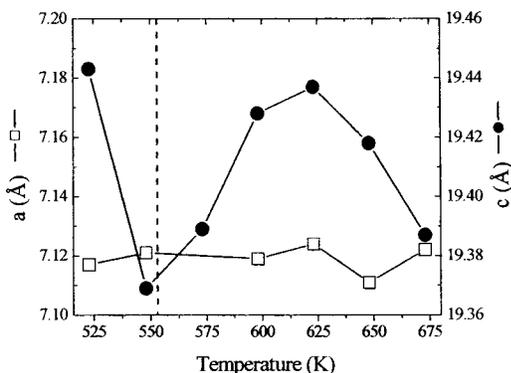
FIG. 4. Variation of the  $a$ - and  $c$ -lattice parameter of  $\gamma$ - $\text{In}_2\text{Se}_3$  thin film according to the substrate temperature. Below a temperature of 560 K, the samples are biphased.
