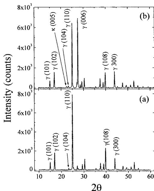
FIG. 5. X-ray diffraction diagrams of undoped  $\gamma$ - $\text{In}_2\text{Se}_3$  (a) and Zn doped  $\text{In}_2\text{Se}_3$  (b) elaborated in the same conditions. Concentration of Zn does not exceed 1 at. %.
