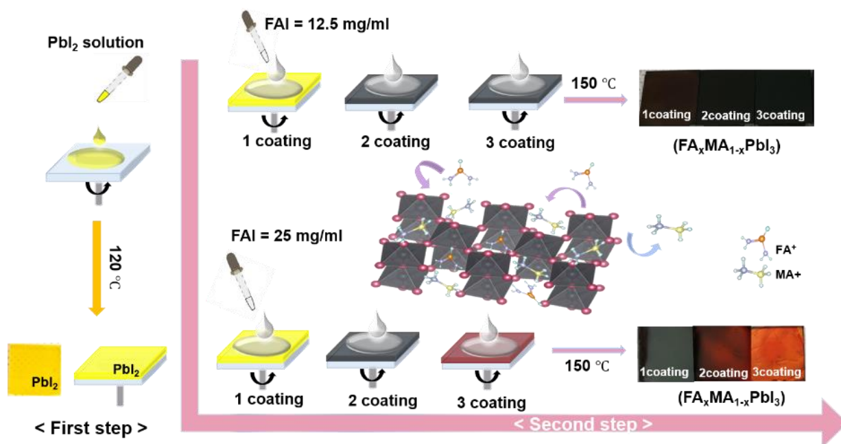
Figure 1. Synthesis of FA_xMA_{1-x}PbI_3 films using mixed FAI–MAI precursors.
