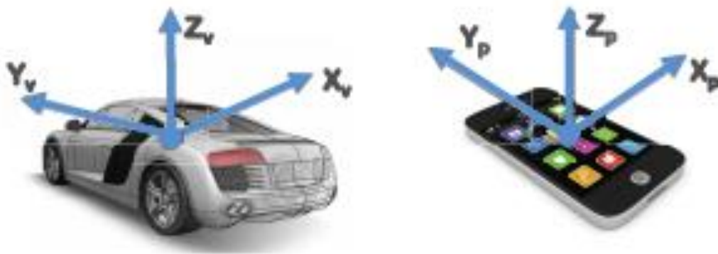
Fig. 11. Vehicle coordinate and smartphone coordinate system [15].
