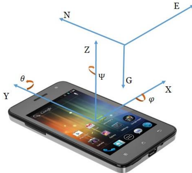
Fig. 18. Smartphone's local coordinate system, global coordinate system and orientation angles made by the phone.
