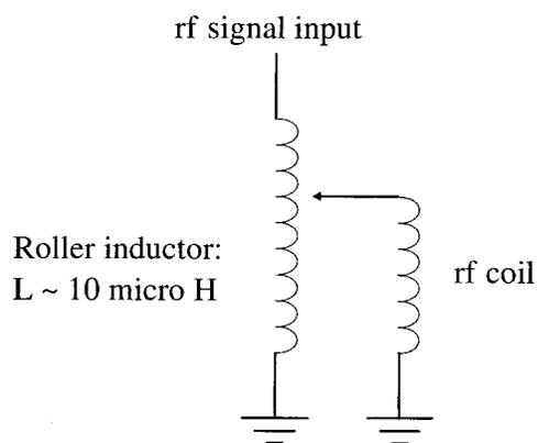
FIG. 2. Schematic of a simple circuit which uses a roller inductor to impedance match the rf source to the cell coil.
