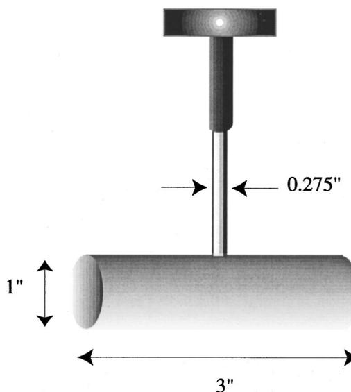
FIG. 1. Sketch of the Pyrex cell used to make a rf discharge in argon.
