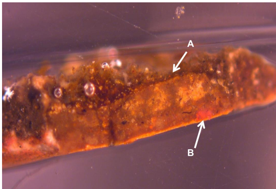
Figure 32. Cross-section of point 4. More discoloration of the copper resinate is shown (A) as well as a large chunk of umber in the paint layer (B).
