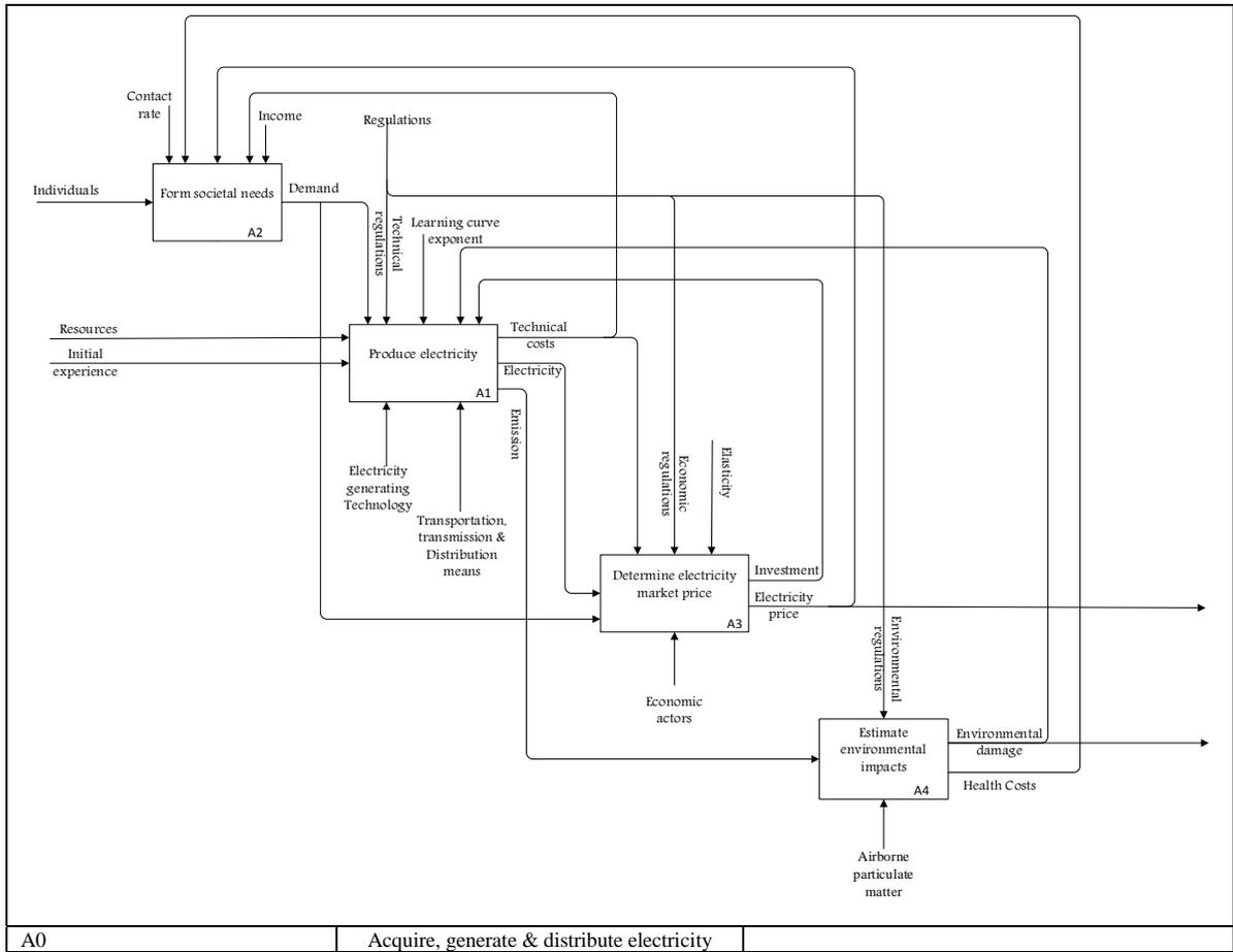
Fig. 2. Graphic diagram of the electricity system
