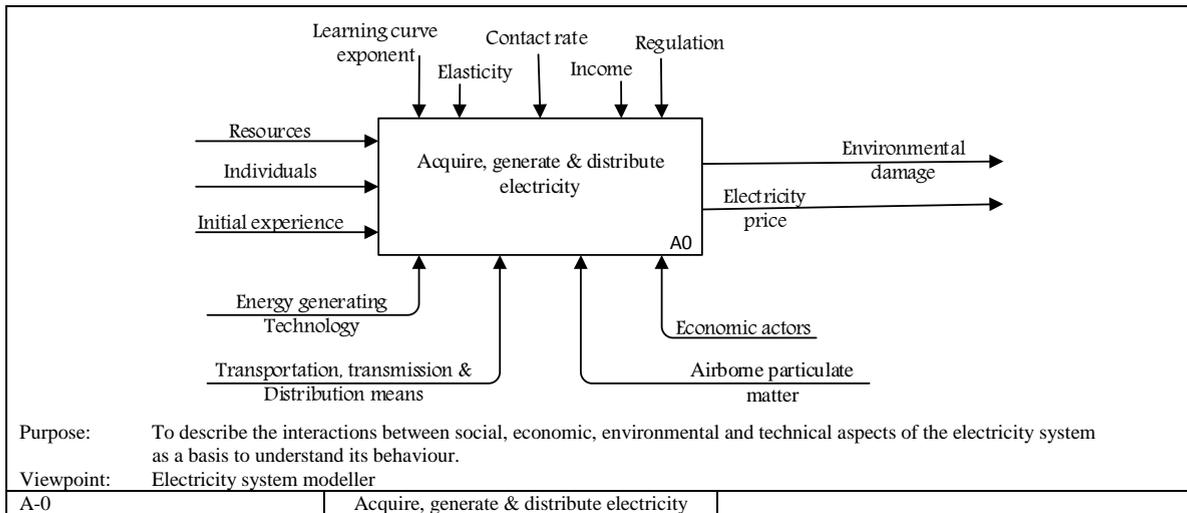
Fig. 1. Graphic diagram of the electrical system, top-level
