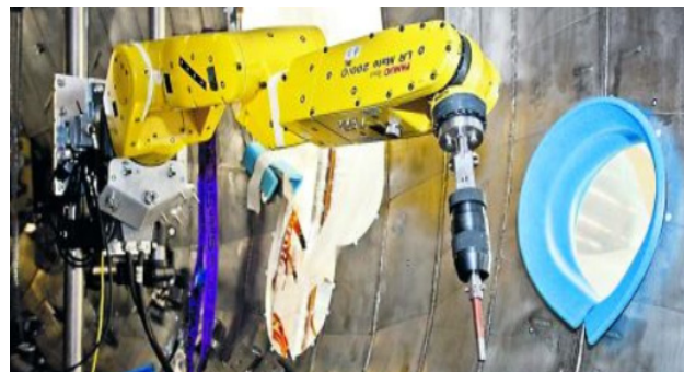
Figure 2 Fanuc LR Mate 200iC in a welding application
