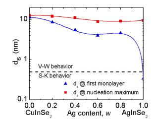
FIG. 2. The surface roughness layer thickness  $d_s$  at the onset of bulk layer formation (i.e., when  $d_b \sim 0.5$  nm) plotted as a function of Ag content w. Also shown is the maximum nucleating or roughness layer thickness during nucleation.
