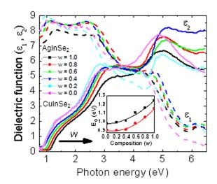
FIG. 3. Dielectric functions for ACIS films of different Ag content *w* deposited at 550 °C. The arrow for  $\varepsilon_2$  (near the band gap) indicates the direction of increasing Ag content. The inset shows the band gap of ACIS at room temperature (squares) and at 550 °C (circles) as a function of Ag content *w*. Polynomial fits (solid lines) provide the bowing parameters.
