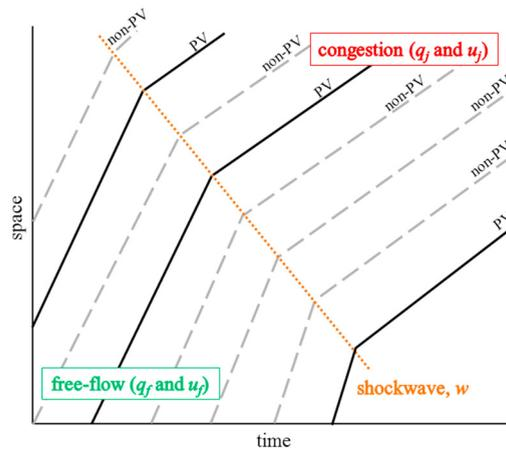
Fig. 1. Sample illustration of trajectory and shockwave
