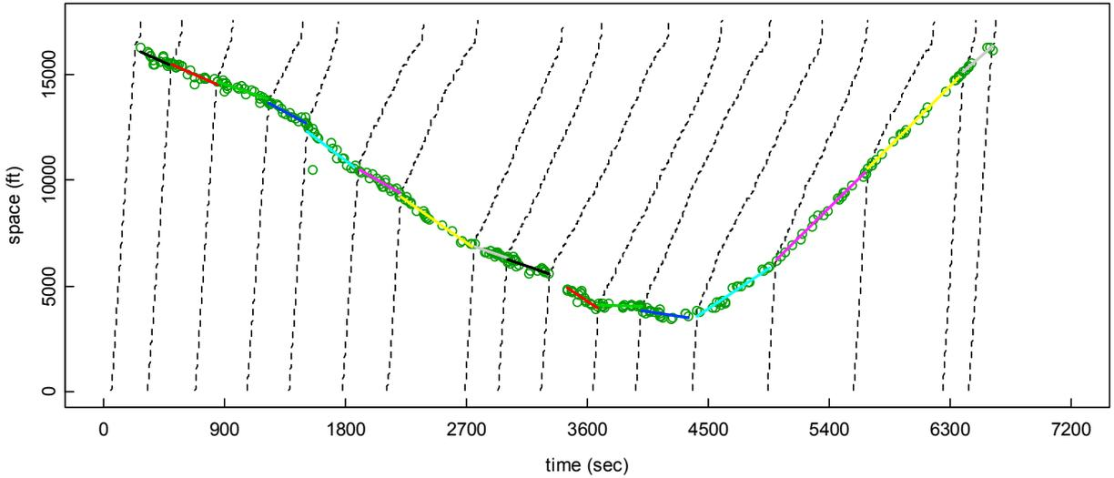
Fig. 4. Probe vehicle trajectory for every 20<sup>th</sup> vehicle, transition points and its shock wave
