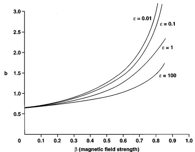
FIG. 3. Plot of displacement thickness  $b$  vs  $\beta$  for various values of  $\epsilon$ . When  $\beta=0$ ,  $b = 0.647900$ .
