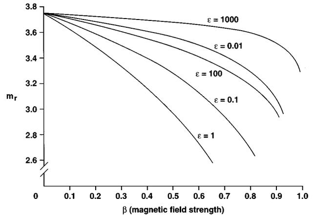
FIG. 6. Plot of slope ratio  $m_r$  vs  $\beta$  for various values of  $\epsilon$ . When  $\beta=0$ ,  $m_r = 3.748\ 513$ .
