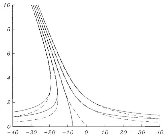
FIG. 7. Graph of streamlines (solid) and magnetic field lines (dashed) near wall for  $\epsilon = 1$ ,  $\beta = 0.4$ .
