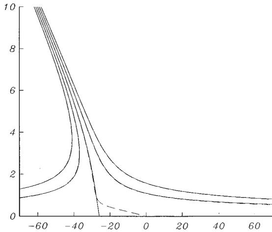
FIG. 8. Graph of streamlines (solid) and magnetic field lines (dashed) near wall for  $\epsilon=100, \beta=0.8$ .
