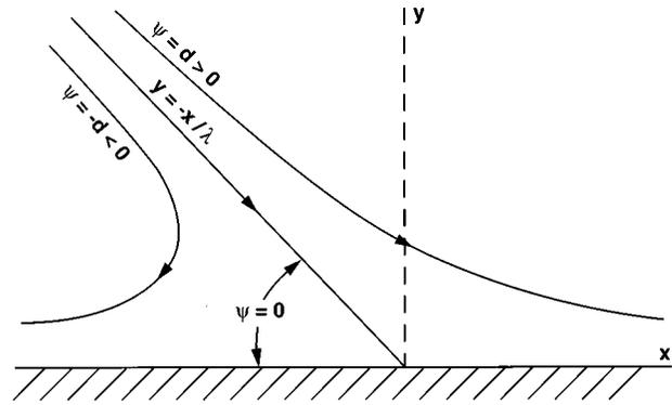
FIG. 4. The undisturbed oblique flow. The dividing streamline has equation  $y = -x/\lambda$ .
