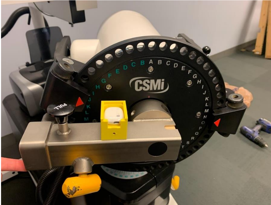
Figure 2. Sensor mounted to dynamometer for bias stability testing.
