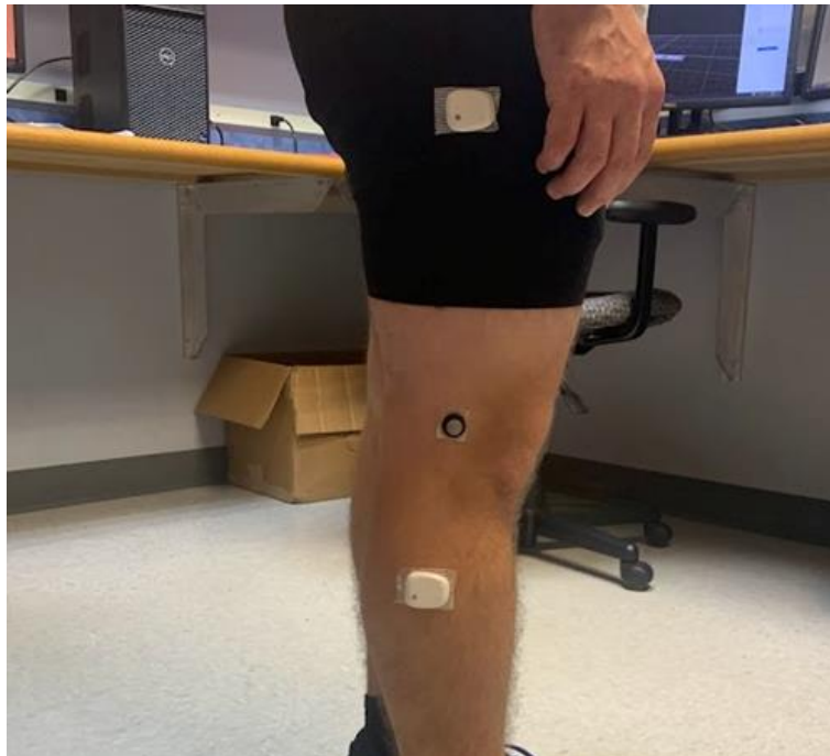
Figure 9. MetaMotion sensor placement on thigh and shank.
