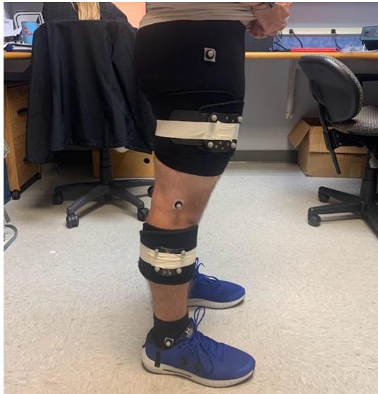
Figure 10. Marker placement guide. Note: MetaMotion sensors are under each marker plate.
