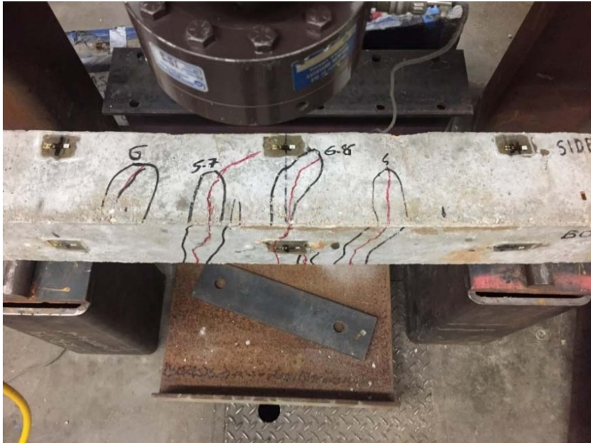
Figure 40. Cracking pattern of Beam 1
