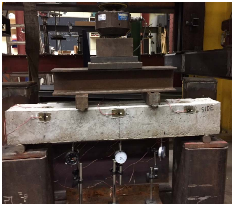
Figure 38. Test Setup for Two-point Load system
