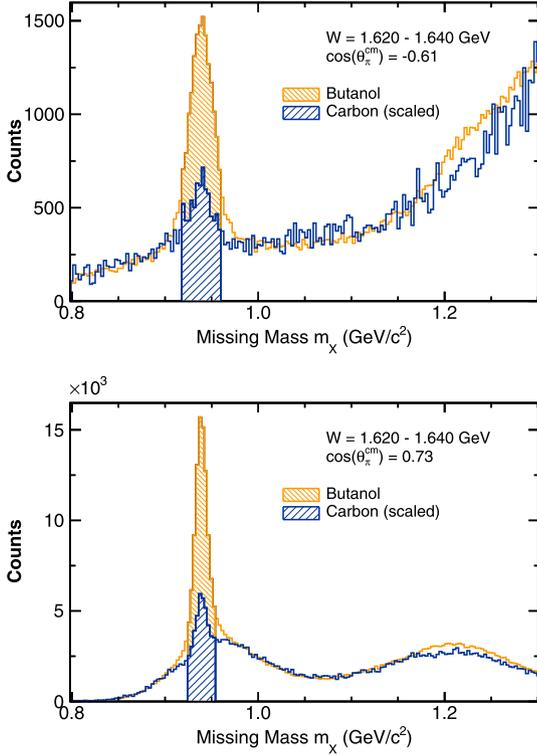
**Fig. 2.** (Color online.) Examples of butanol missing-mass distributions,  $\gamma p \rightarrow \pi^+ X$ , overlaid with scaled distributions from the carbon-target. The hatched region selects the butanol- and carbon-target events which were used in the subsequent analysis. The butanol yield at larger missing masses contains multi-pion final-state events off the free proton and exceed the carbon yield.
