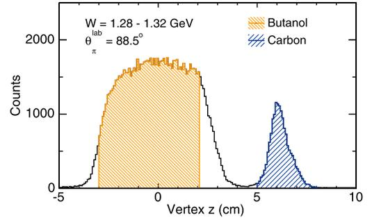
**Fig. 1.** Example of a reconstructed distribution of the reaction vertex along the beam line for events at  $W \approx 1.30$  GeV and  $\theta_{\pi}^{\text{lab}} \approx 88.5^\circ$  originating in the butanol and carbon targets. The shaded areas indicate the  $z$ -vertex ranges used in the analysis.
