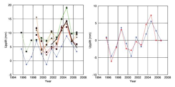
Figure 6. Measured and predicted yearly uplifts. Left: Time-series for the individual solutions. The stations are—stars: NYA1; squares: NYAL; circles: VLBI. The solutions are—green: GIPSY–PPP; red: GAMIT; orange: GIPSY–REG, black: VLBI. In blue, the predicted uplift is shown (for the ice model, see Table 5). Right: mean of the annual displacements after the individual biases have been removed (in red) and the predicted annual displacements (in blue, mean has been removed).
