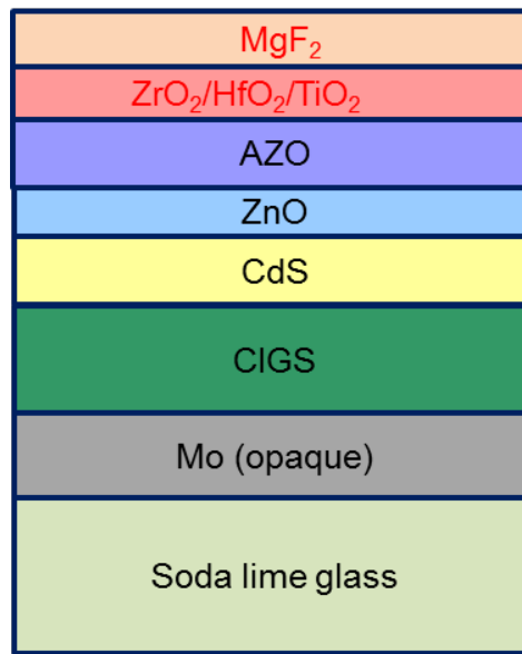
Figure 5. 1: Schematic diagram of ultra-thin CIGS solar cell with 2-layer ARC.
