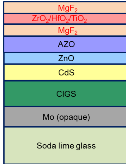
Figure 5. 9: Schematic diagram of ultra-thin CIGS solar cell with 3-layer ARC.
