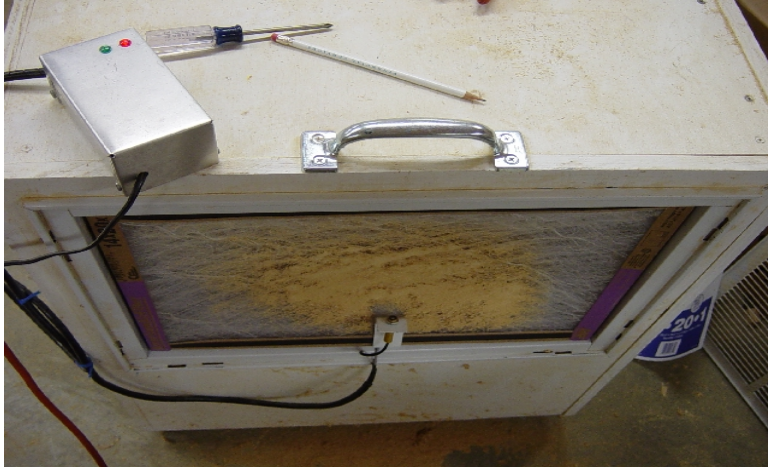
Figure 6. Air-Filter with a Red LED On When Sensing Light Is Blocked
