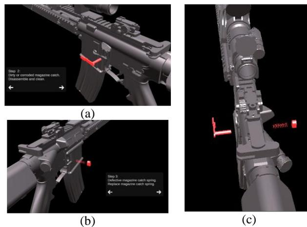
Figure 2. (a) Screenshot of step 2 of the failure of the magazine to lock procedure. (b) Screenshot of step 3 of the failure of the magazine to lock procedure. (c) Screenshots of the transition from step 2 to step 3.
