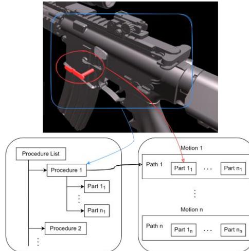
Figure 1. Mapping relations of operation procedure and virtual model
