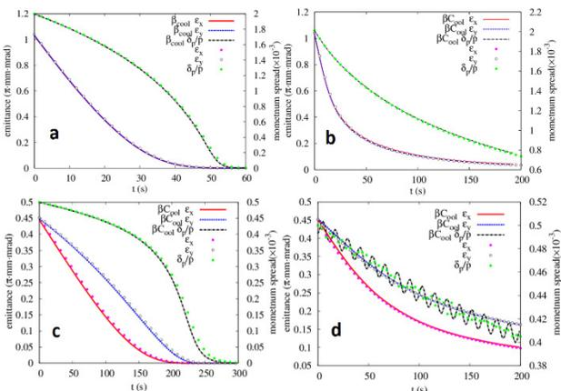
Figure 4: Emittance shrink due to electron cooling.
