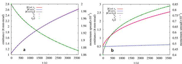
Figure 3: Emittance expansion due to IBS effect.
