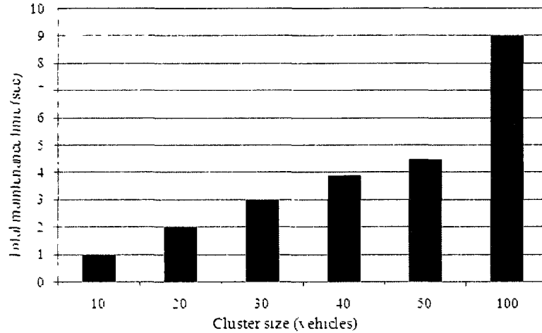
FIG. 26: Impact of cluster size on cluster maintenance time
