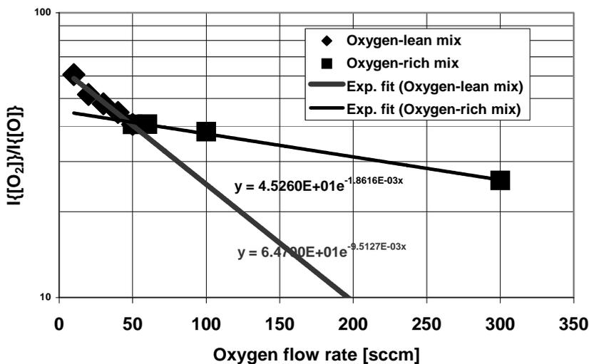
**Figure 6.** Ratio of molecular ion band integral intensity ( $^4\Sigma_g^- \rightarrow ^4\Pi_u$  system) to the atomic line ( $^5P-^5D^0$ ) intensity at Helium flow rate of 3000 sccm.
