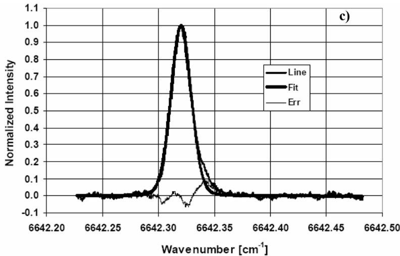
**Figure 2.** c) Absorption line profile of Q(4) at 300 sccm flow of oxygen and 3000 sccm flow of helium. Discharge parameters:  $E/N = 20.76$  Td,  $p = 16.1$  Torr,  $T = 550$  K. Ratio of Lorentz to Voigt profile  $\Delta\omega_L/\Delta\omega_V = 0.11$  indicates dominant temperature (Doppler) broadening mechanism. Central wavenumber  $\omega_0 = 6642.3202$   $\text{cm}^{-1}$ . Fitting error  $\sim 2\%$ .
