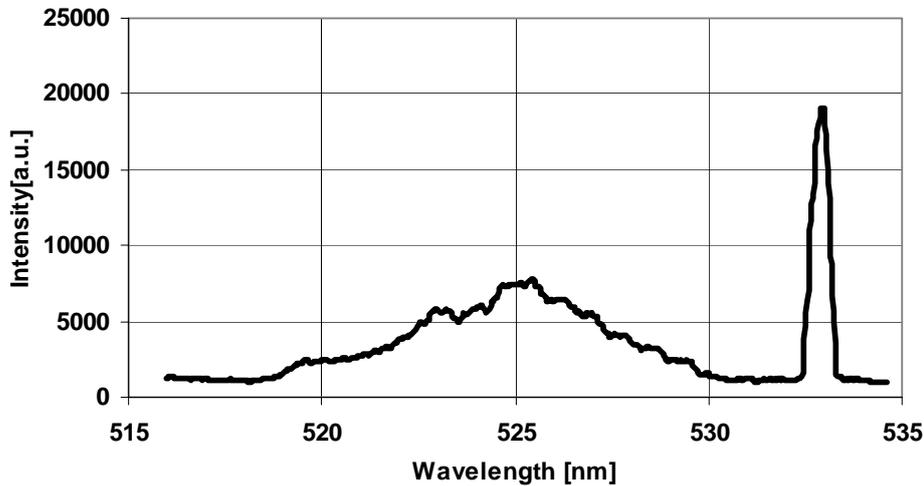
**Figure 5.** Spectrum of the He/O<sub>2</sub> discharge showing simultaneous emission of a system of molecular oxygen ion bands from the  $^4\Sigma_g^- \rightarrow ^4\Pi_u$  system around 520 nm, and the  $^5P-^5D^0$  atomic oxygen emission at 533.07 nm.
