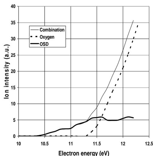
**Figure 1.** Threshold ionization curves from a Wood's discharge: discharge off, thin solid line; discharge on, dashed line; OSD, thick solid line.
