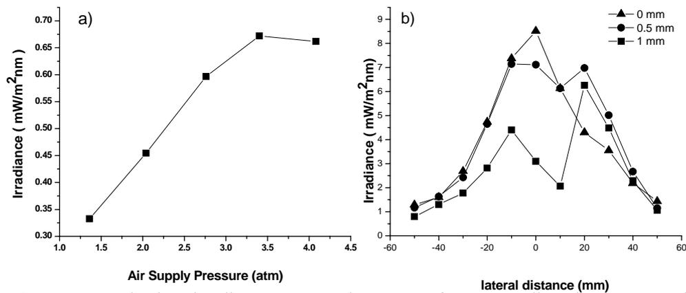
**Figure 8.** Average absolute irradiance over torch segment for oxygen lines in the spectral region between 777.1 and 777.6 nm dependence on: a) air supply pressure for 2 mm above the surface of waveguide, b) spatial position.
