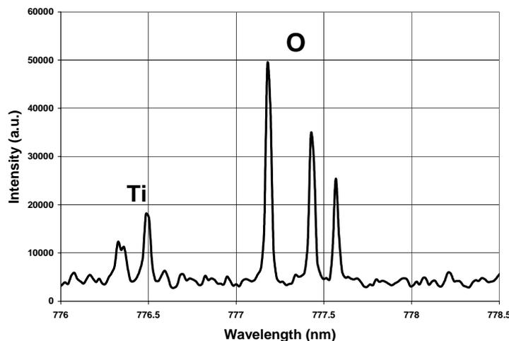
**Figure 7.** Emission spectrum in the region from 776 – 778.5 nm emitted from the torch at 2 cm above the surface of the waveguide.
