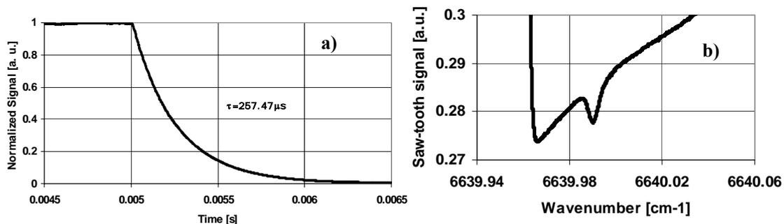
**Figure 2.** a) Measured ringdown decay signal. The ringdown time  $\tau = 257.47\ \mu\text{s}$  is obtained using the exponential fit of the decay signal between 0.1 and 0.9 with an error less than 0.1%;
