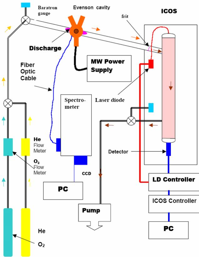
**Figure 3.** Schematic diagram of OSD production and detection apparatus.
