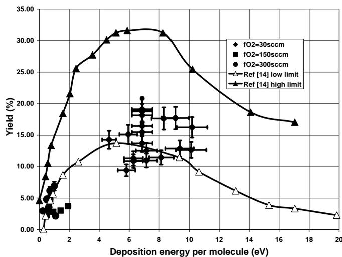
**Figure 4.** OSD yield as a function of specific energy deposition in Oxygen molecules. Solid lines: envelopes of the factorial computational experiment data of Ref. [14]. Error in present experimental data is due to uncertainties in electron and gas-kinetic temperature, and estimated uncertainty of constant field approximation.
