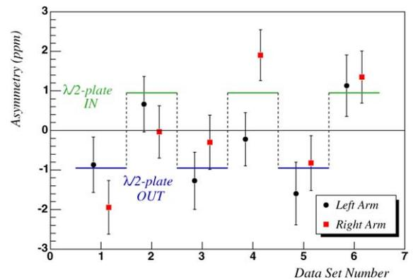
Fig. 1.  $A_{\text{raw}}$  for all data, grouped by  $\lambda/2$ -plate state in 6 sequential data sets. The circles and squares represent the average of the 2 PMT channels in each spectrometer arm, and the line represents  $A_{\text{raw}}$ , averaged over the run and plotted with the appropriate sign for each half-wave plate state.
