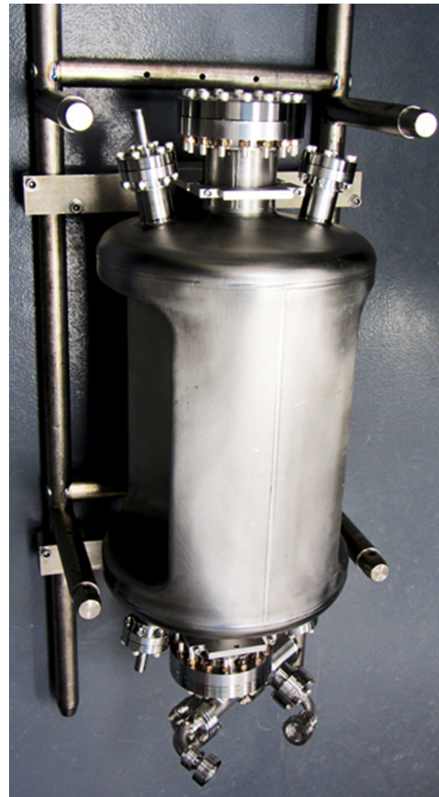
FIG. 8. Assembled cavity prior to test with fixed input coupler at the bottom and pickup probe at the top.
