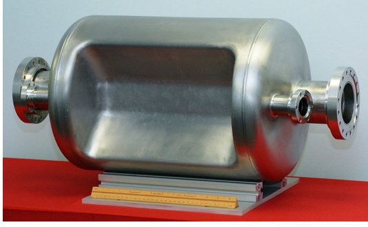
FIG. 4. Fabricated 400 MHz rf-dipole cavity.
