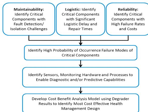
Figure 1. Degradation Analysis, adapted from [12]
