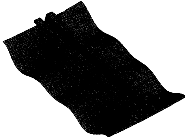
Figure 4. Local skin buckling mode for hat-stiffened panel
