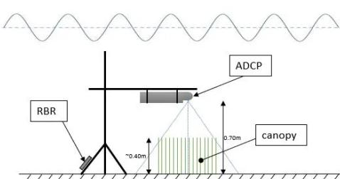
Figure 2: Instrument setup in the field.
