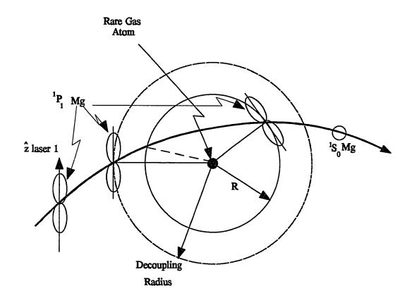
Adiabatic reorientation of the 3p  $\Sigma$  level probed to the 4d  $\Sigma$  level during a collision. *R* represents the Condon point for the laser 2 detuning.
