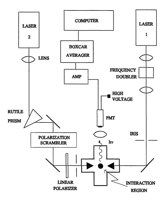
FIGURE 16 Schematic diagram of the apparatus used for experiment B.
