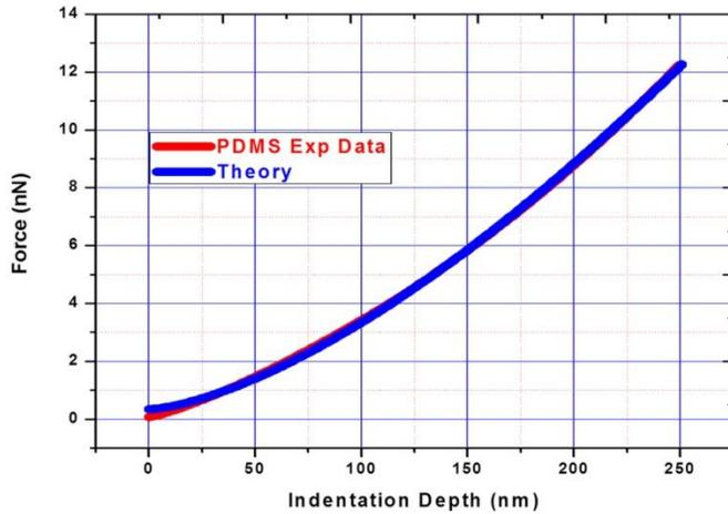
**Figure 3.** Force-indentation measurements of PDMS using force spectroscopy mode atomic force microscopy.
