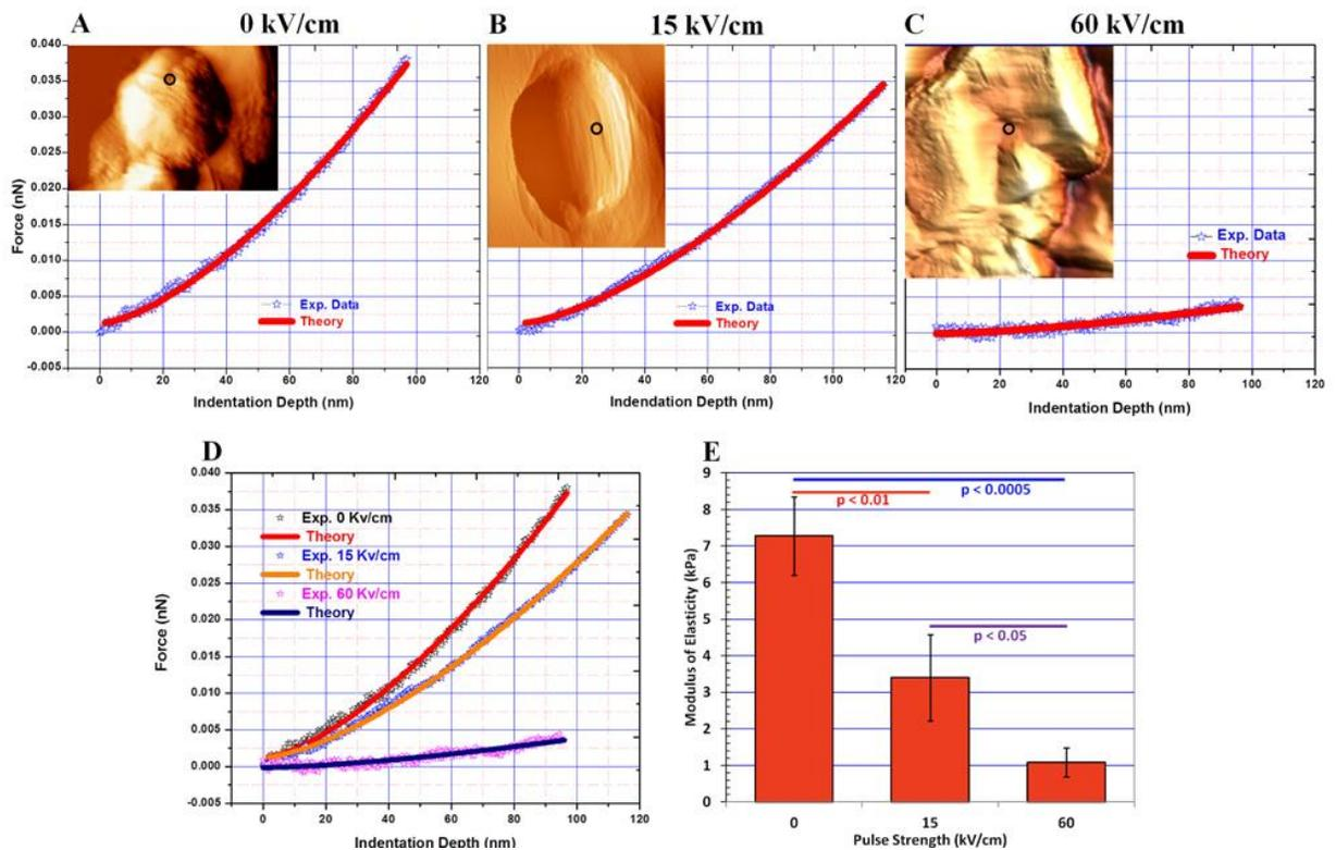
**Figure 4.** Young's modulus of Jurkat cells exposed to nanosecond pulsed electric fields (nsPEFs) using force spectroscopy mode atomic force microscopy (FS-AFM). Membrane force-indentation measurements of cells exposed to (A) 0, (B) 15, and (C) 60 kV/cm nsPEFs using FS-AFM. The black circles mark the point on the cell where force measurements were taken.
