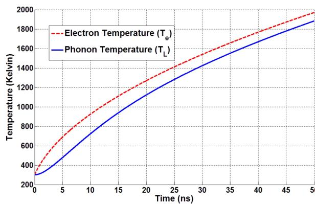
FIG. 3. Simulation results showing the temporal evolution of the temperatures for electrons and ( $5 \times 10^7 \text{ m}^{-1}$  wavevector) phonons at an electric field of  $4 \times 10^3 \text{ V/m}$ .
