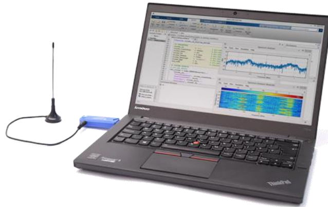
Figure 7 A Lenovo Thinkpad laptop computer with RTL-SDR USB Dongle attached. [ http://www.desktopSDR.com/hardware , Dec 22, 2016.]
