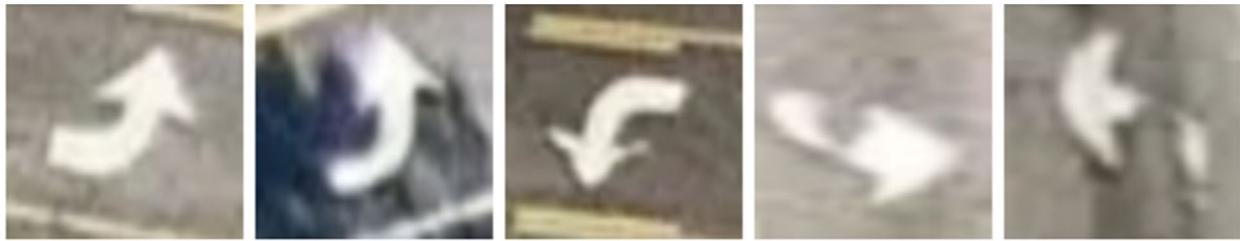
(a) Correctly classified lane-use arrows (Ground truth: High, High, High, Low, Low; Predict: High, High, High, Low, Low)
