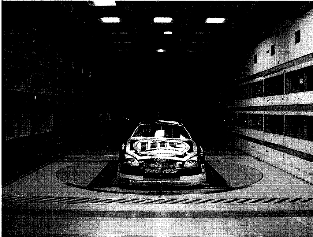
Figure (5.1) Vehicle in closed wall test section
