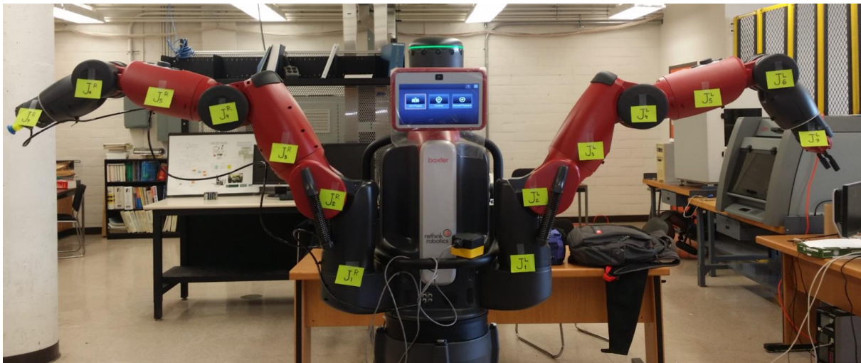
Figure 8: Baxter cobot left and right joints
