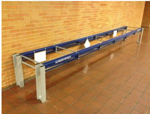
Figure 1. Model Steel Bridge
