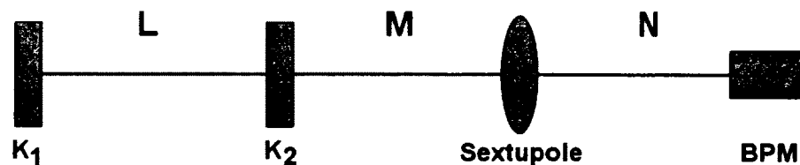
FIG. 13. A simple model of beamline elements for demonstrating how two distinct frequencies of a simultaneously modulated electron beam will mix due to the non-linear fields of a sextupole.
