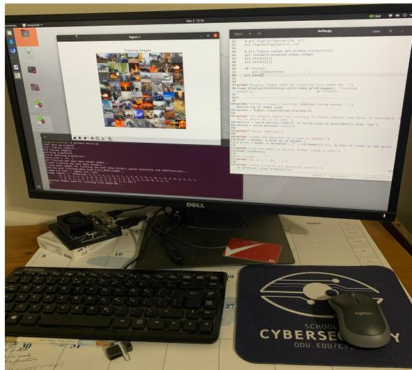
Figure 8: Jetson Nano configured and running the Fire-Smoke Classifier CNN.
