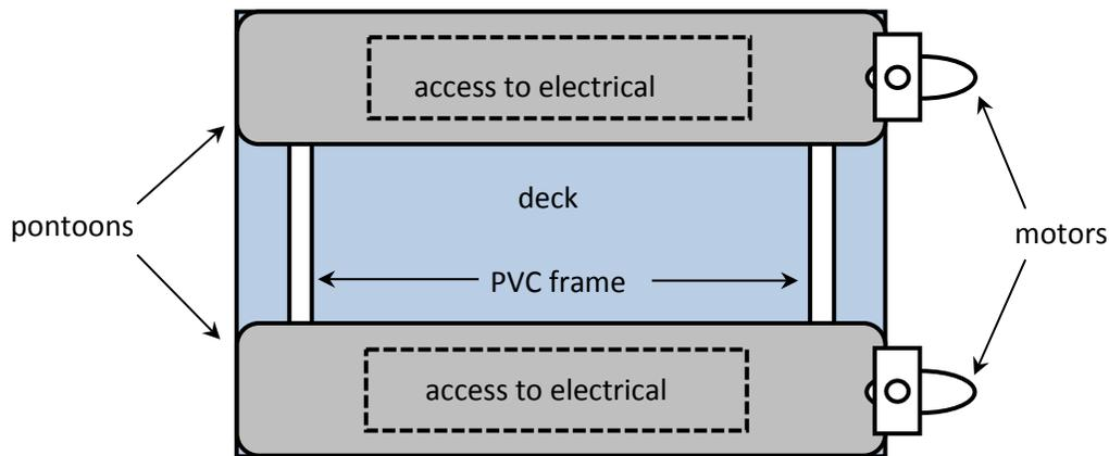
Figure A.6. Bottom view of proposed hull layout. Access to the electrical housing in the pontoons is through an access panel on top of the deck (dashed lines in figure).
