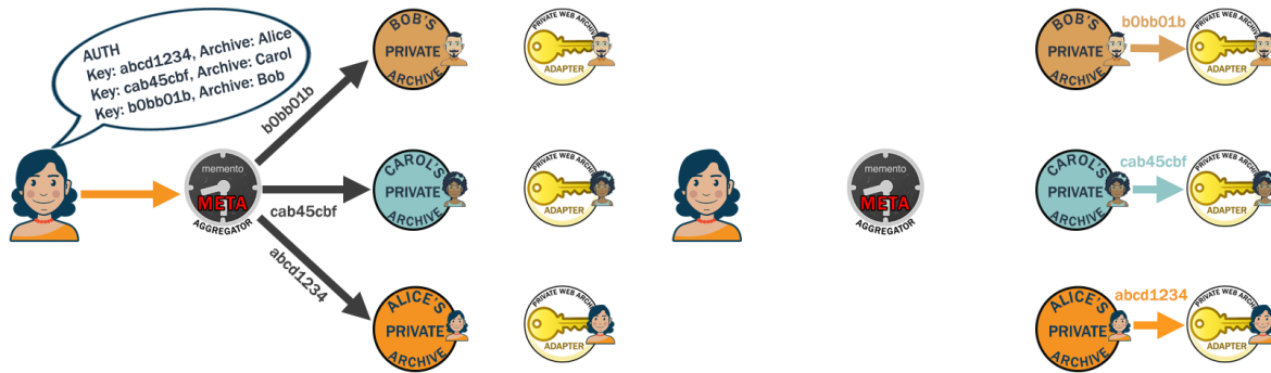
(a) A user provides different keys for three different private Web archives, aggregated by an MMA
