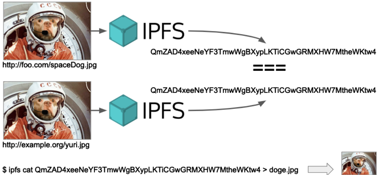
Fig. 38 Content addressing entails generating a hash of a file and using that hash as a means up retrieving the content. Two identical images at different URIs will result in the same hash when content addressing and identical hashing algorithms are used. In IPFS, this hash can be used for retrieving the image instead of retrieving the image by URI.
