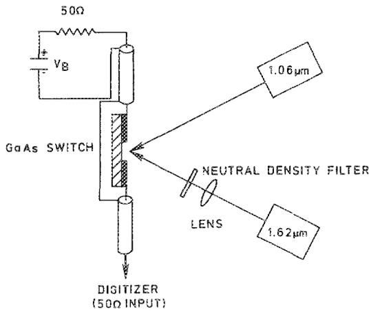
FIG. 1. Diagram illustrating the experimental setup. Note that the crystal was illuminated on the face containing the contacts.
