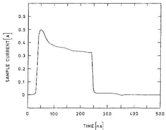
FIG. 3. Measured current flowing through the *p*-type crystal. Sample conductivity is induced initially by the  $1.06 \text{ } \mu\text{m}$  laser pulse. The sample conductivity is quenched 200 ns later by the  $1.8 \text{ } \mu\text{m}$  laser pulse. The initial bias voltage is 55 V.
