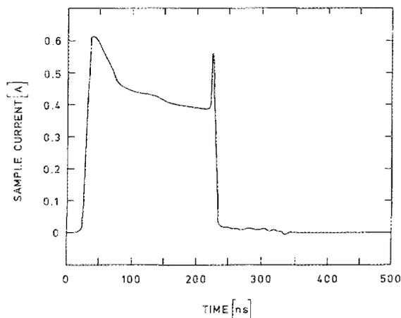
FIG. 2. Measured current flowing through the *p*-type crystal. Sample conductivity is induced initially by the  $1.06 \text{ } \mu\text{m}$  laser pulse. The sample conductivity is quenched 200 ns later by the  $1.62 \text{ } \mu\text{m}$  laser pulse. The initial bias voltage is 67 V.
