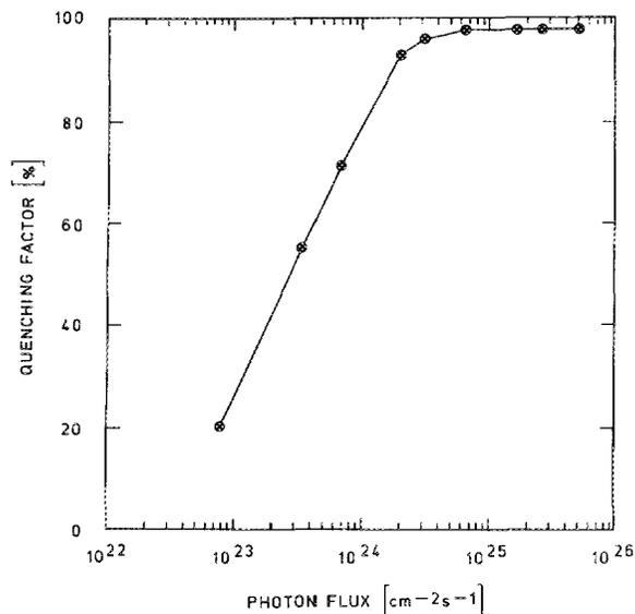
FIG. 4. Quenching factor as a function of the  $1.62\ \mu\text{m}$  laser pulse peak intensity. The maximum quenching factor that could be resolved was 98%.
