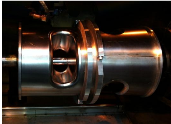
Figure 4: Cavity main body middle seam welding.
