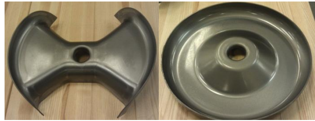
Figure 1: Formed spoke half and end cap.
