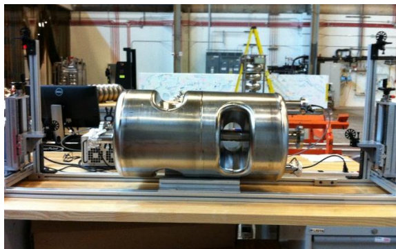
Figure 5: Complete cavity for bead pull set up.
