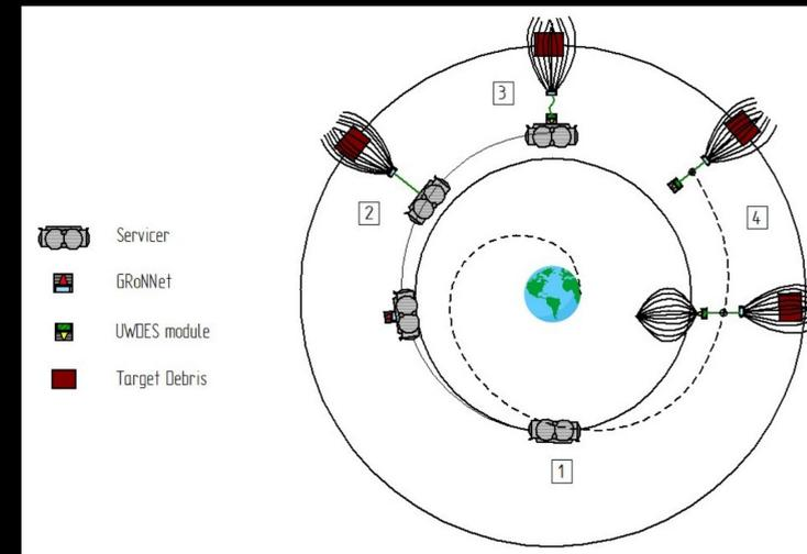
Figure 3. Mission CONOPS – (1) Host S/C Orbit Insertion, (2) GRoNNet Module Deployed, (3) GRoNNet Captures Target Debris, (4) UWDES or mDEMS is Deployed for Expedited Re-entry of Target Debris
