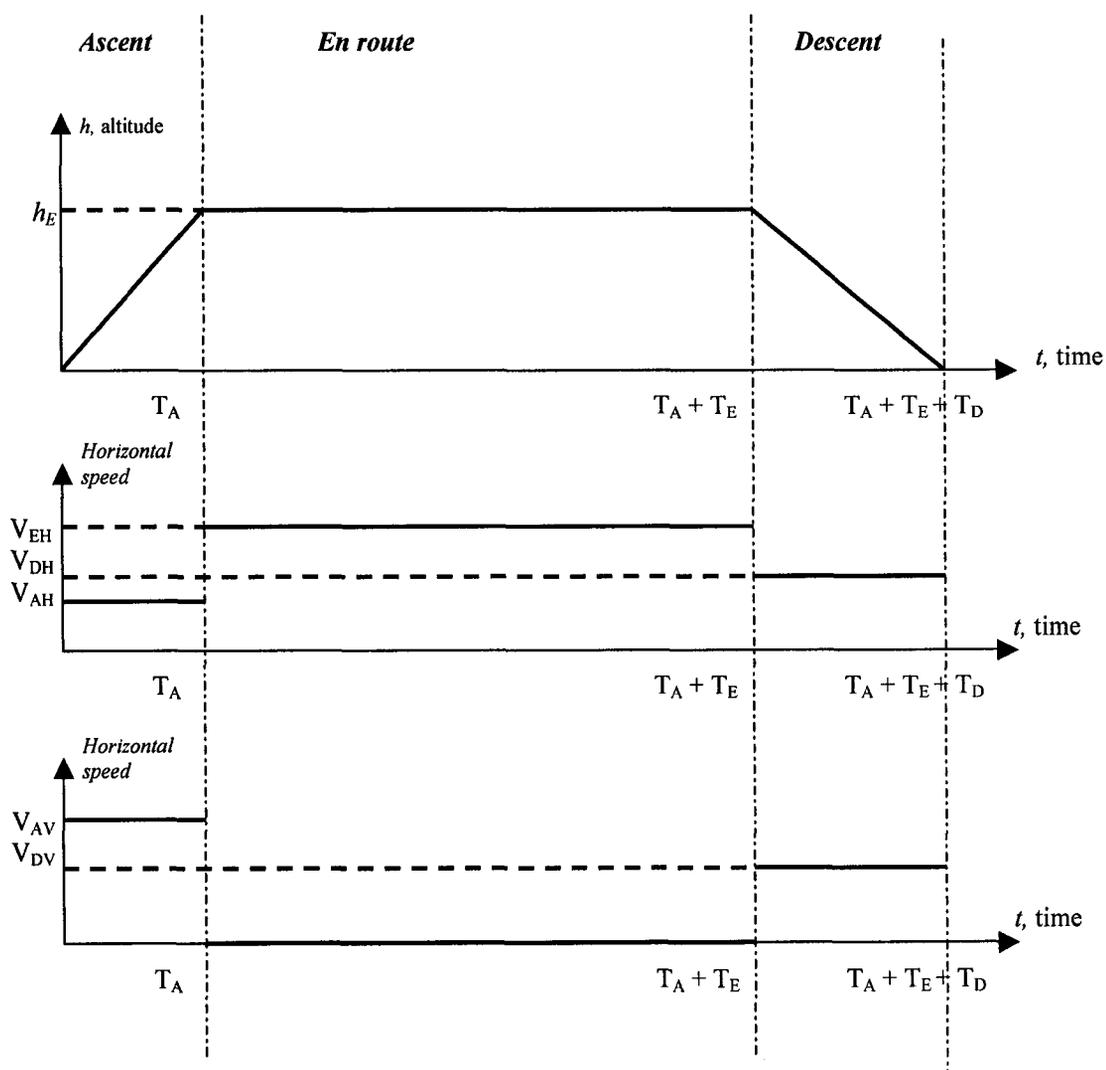
**Figure 9** Altitude, horizontal and vertical aircraft speed characteristics.
